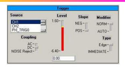
**Source:** The trigger source for the digitizer may be either of the input channels or the PXI Trigger and Star Trigger lines on the PXI backplane.
