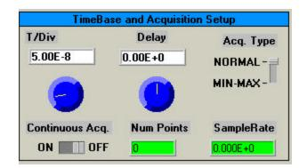
**T/Div:** The time per division is set by using the **T/Div** knob or by typing a value in the T/Div control box. The digitizer automatically adapts itself to use the maximum sampling rate whenever the timebase is changed.
